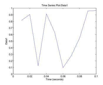
Notice how the object's plot function creates a graph that is plotted and labeled with the data from the tsobj object. As a user of this object, you do not need write your own code to produce this graph. The class design specifies the standard way to present graphs of timeseries data and all clients of this object use the same code for plotting.
