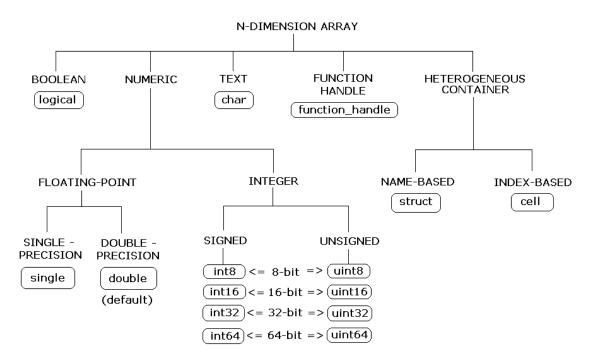
Numeric classes in the MATLAB software include signed and unsigned integers, and single- and double-precision floating-point numbers. By default, MATLAB stores all numeric values as double-precision floating point. (You cannot change the default type and precision.) You can choose to store any number, or array of numbers, as integers or as single-precision. Integer and single-precision arrays offer more memory-efficient storage than double-precision.
